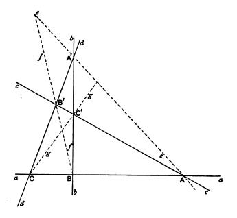
the points ac, bd are a pair of opposite vertices, and the line joining them, denoted by e in the figure, is a diagonal. If A, A'; B, B'; C, C'; be the three pairs of opposite vertices, the lines of the tetragram are ABC, AB'C', A'BC', and A'B'C.
